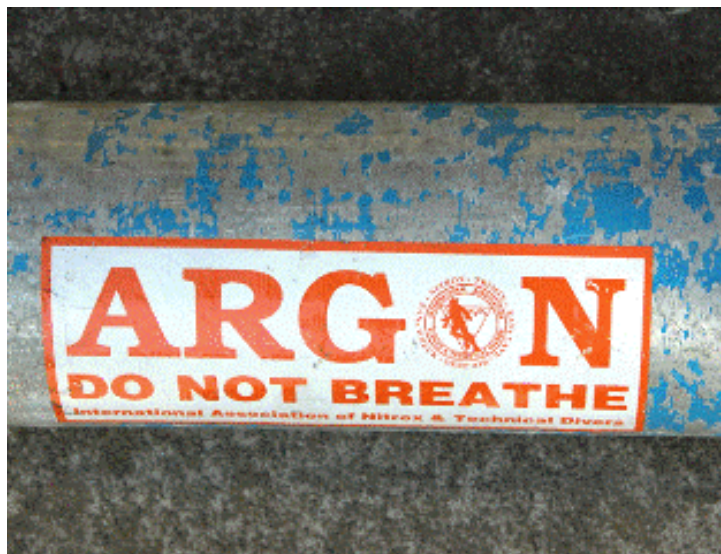
Figure 6 Clear tank markings, dedicated tank service, repeated analysis of gas composition and pressures are all key components for enhancing the safety of mixed gas diving.
