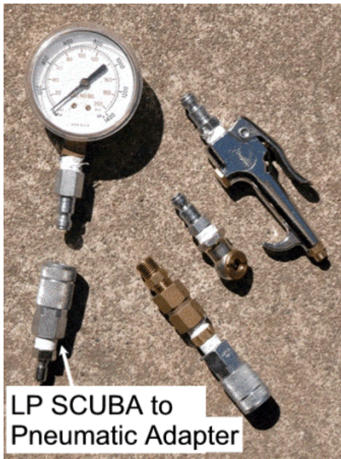
Figure 2 A pressure gauge, coupled to a standard industrial pneumatic fitting, is used to adjust the inflation regulator's interstage pressure and also the pressure relief valve's blow-off pressure. Other fittings are shown as examples of other convenient utilities that can be hooked-up to SCUBA for purposes such as lift bag inflation, or driving a booster pump.
