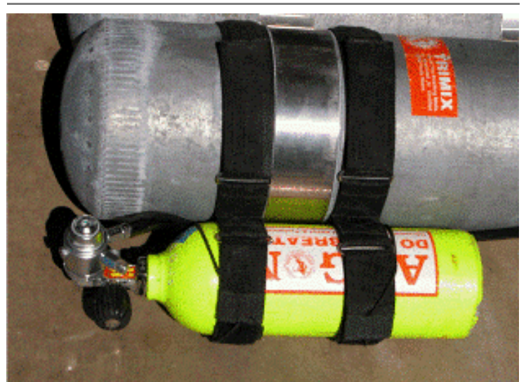
Figure 5 A large tank-mounted pony bottle is not as streamlined as a small bottle fixed to the back plate. Nonetheless, one fill supports multiple dives and even a very low pressure partial fill will be adequate for a long decompression dive.
