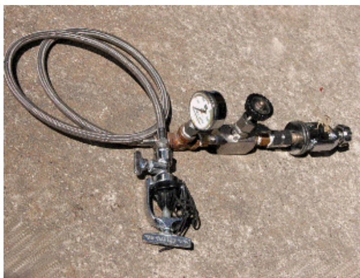
Figure 3 DIY O 2 -Clean gas transfer whip. Stainless steel fittings are used for components that are changed frequently.
