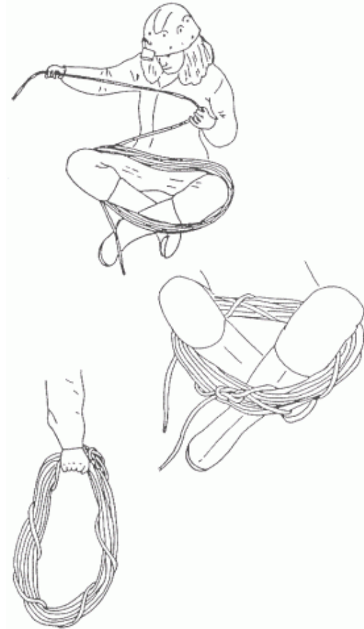
Rolling a rope - wagon wheel
