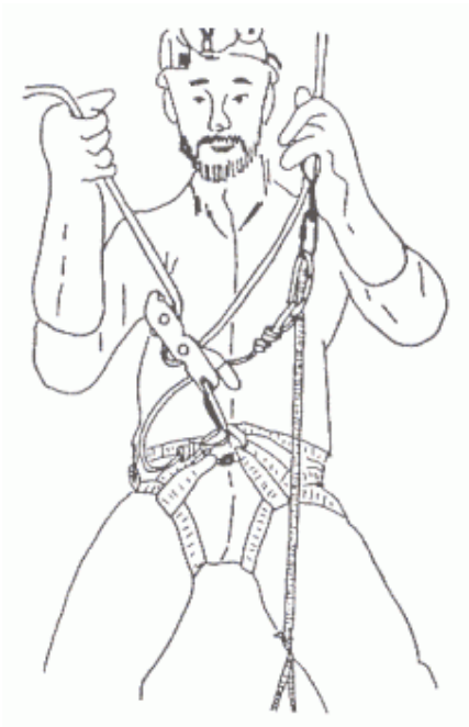
Climbing with one ascender and an autostop
