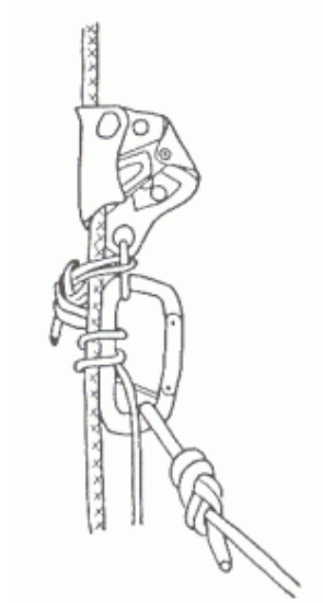
Ascender rigged for muddy rope
