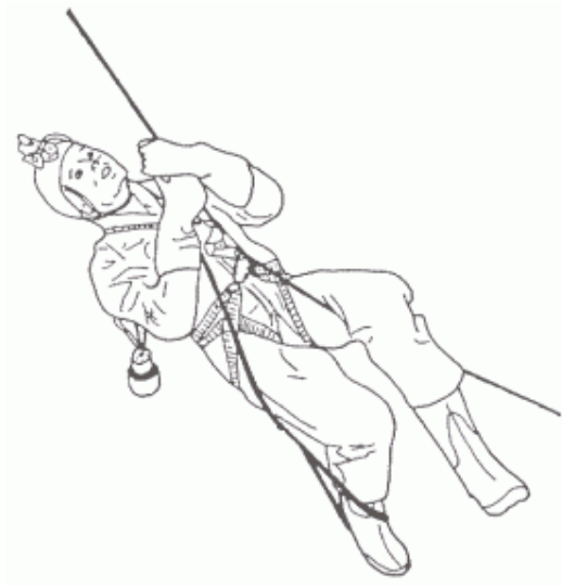
Prusiking a diagonal rope
