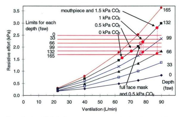
**Figure 11.** How CO<sub>2</sub> in the inspired gas influences a diver breathing on a UBA with a mouthpiece (red, filled circles) and a full face mask with a well-fitting oronasal cup (red, open circles). Horizontal lines show the proposed limits for resistive effort for each depth. Data are from Figure 5.
