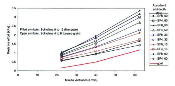
**Figure 7.** Resistive effort data from one MK 25 UBA plotted against minute ventilation. The current NEDU performance goal is also shown. The MK 25 was tested with two absorbents at depths down to 60 fsw (about 18 msw). In the legend, "SF8" refers to Sofnolime 812<sup>®</sup> and "SF4" refers to Sofnolime 408<sup>®</sup>; the numbers "00" through "60" refer to the depth.
