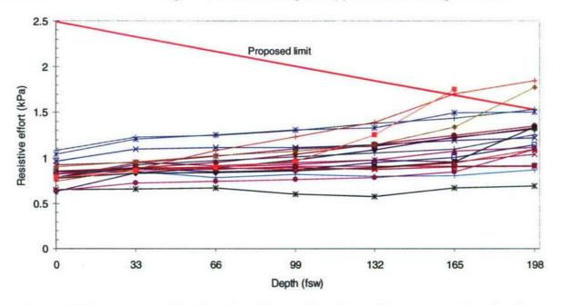
**Figure 4.** The proposed limit and resistive efforts from 20 regulators breathed at 62.5 L/min. The statistical analysis has been omitted for clarity.
