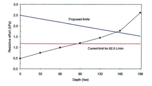
**Figure 6.** Current performance goal and the proposed limit are plotted together with actual data from one MK 16 MOD 1 tested in the prone position with a minute ventilation of 62.5 L/min.
